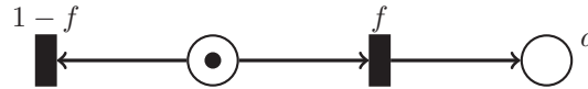
Figure 2: Two transition model of the failure of the blocking mechanism of anchorage a .
