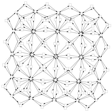
Graphical representation for D = 5, generated by unfolding and automatic layout of a coloured Petri net using Snoopy.
